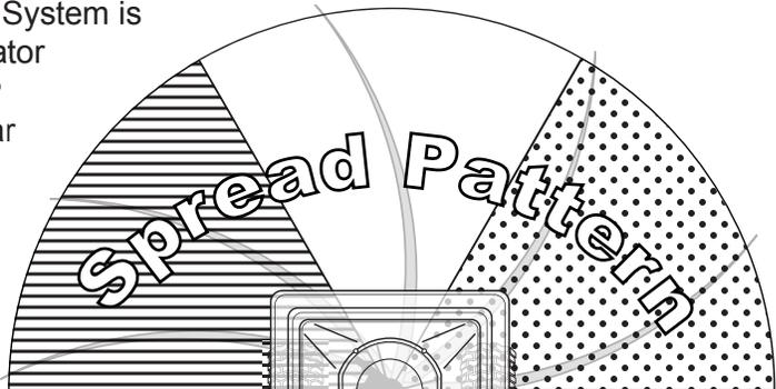
**Adjustable Throwing Ports with 8 repeatable settings to balance the left or right spread pattern to the center.**
