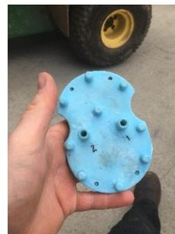
4. Place the pump on a flat work surface and undo the silver plate or bolt using an 8mm spanner. Then undo all the 8 Phillips screws the pump should then come apart. (pictures 7, 8 and 9 **note** The white pump has a silver pressure plate and the blue a single bolt)
