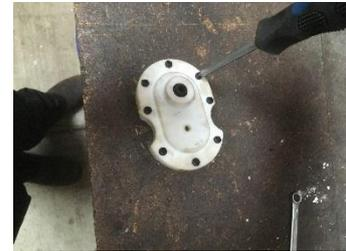
5. Thoroughly wash the 2 gears and the gear casing, hot soapy water is best. If you have some grease available greasing the black O ring seal before reassembly is beneficial. (pictures 10, 11, picture 12 showing after cleaning)
