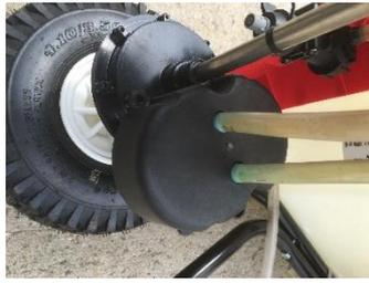
Fill the tank with at least 10 litres of clean water and run through the pump and spray out of the nozzle. It will be easier to remove the nozzle to begin with to speed up this process. This rinse will thoroughly clean the pipes. **Note.** The sprayer maybe hard to push initial if there is further debris from the pipes going through the pump, but it should free up as any remaining debris is exited at the nozzle
