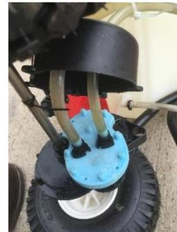
2. Undo the two black zip clips holding the two pipes onto the pumps moulded hose tail ends. These are easily undone by using a flat head screw driver to get behind the clips and ease them off. Keep the clips safe for reconnecting the pipes. (*picture 4*)
