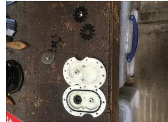
6. Reassemble the gears and casing, relocating and tighten the 8 screws first followed by the silver pressure plate or the bolt. Do not overtighten the plate S25 or the bolt on the S15 Ensuring the gears are in the correct position and the two halves of the casing are correctly aligned, the two bevels together as in the below (picture 13)
