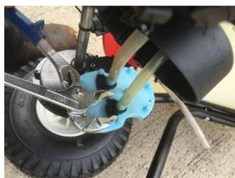
8. Relocate the pump case cover with the 3 Phillips screws. *(picture 16)*
