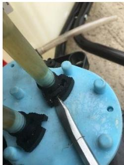
3. Pull the pipes off the moulded hose tails you may need to twist them as you pull, to ease them off. **IMPORTANT** Make sure you note which pipe goes to each hose tail so you replace them in the correct order. (*see pictures 5 and 6 and 7, note pipe and pump can be marked with a felt pen for easy reassembly as shown*)
