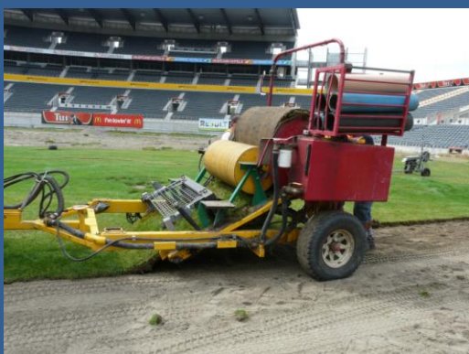
Harvesting turf from AMI Stadium for recycling at the Christchurch Temporary Stadium, Addington.
